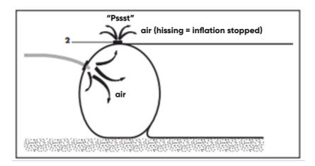
5. Stop the inflation device, remove the nozzle of the device from the water connection.
