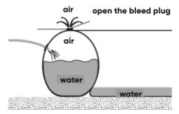
4. The skirting is full of water when it escapes from the pressure relief valve(s). Stop filling and remove the hose.
