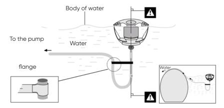
As it floats freely on the water, this floating skimmer has the advantage of automatically adjusting itself in relation to the body of water.
