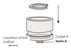
4. Check that the body is properly engaged in the float unit, place the pre-filter basket in the body, then place the float on the body.
