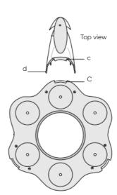
3. Place the ballast in the body of the skimmer and screw the barbed connector to the skimmer outlet.
